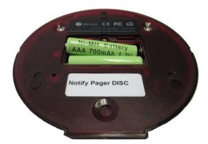
**User replaceable battery (URB)** There is no need to return the pagers, to the supplier for simple battery changes.
